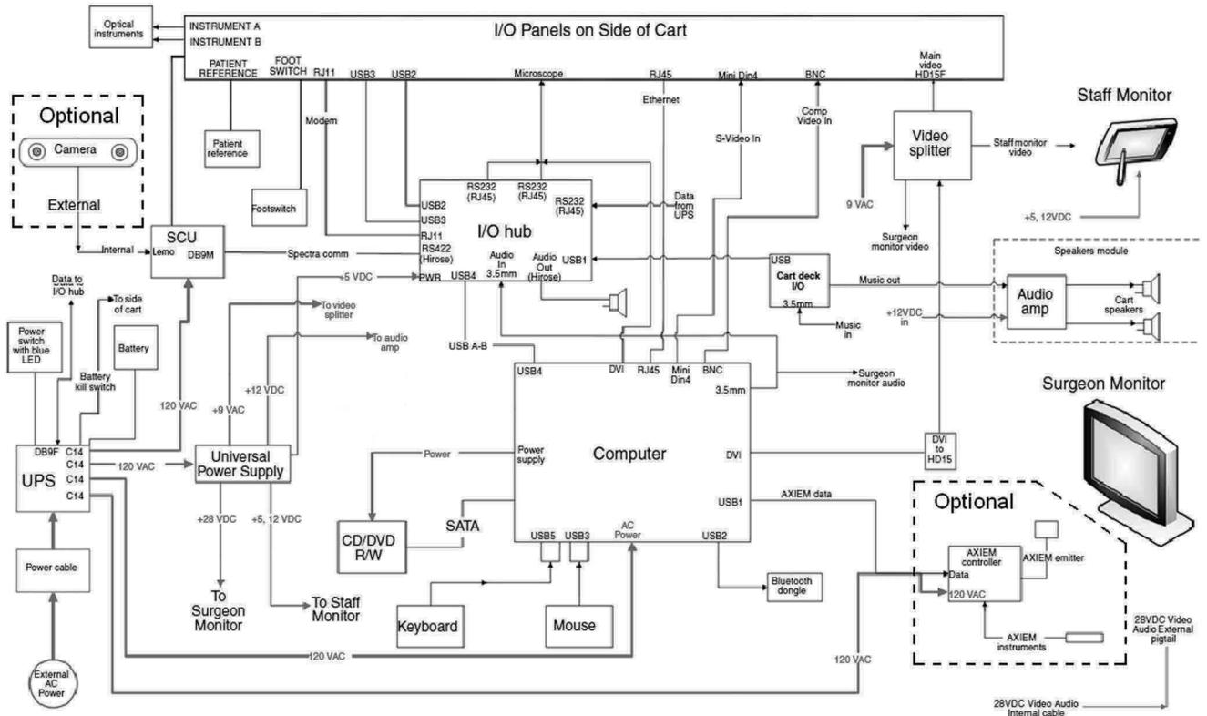
Figure 5-5. Component connections (computer A)
