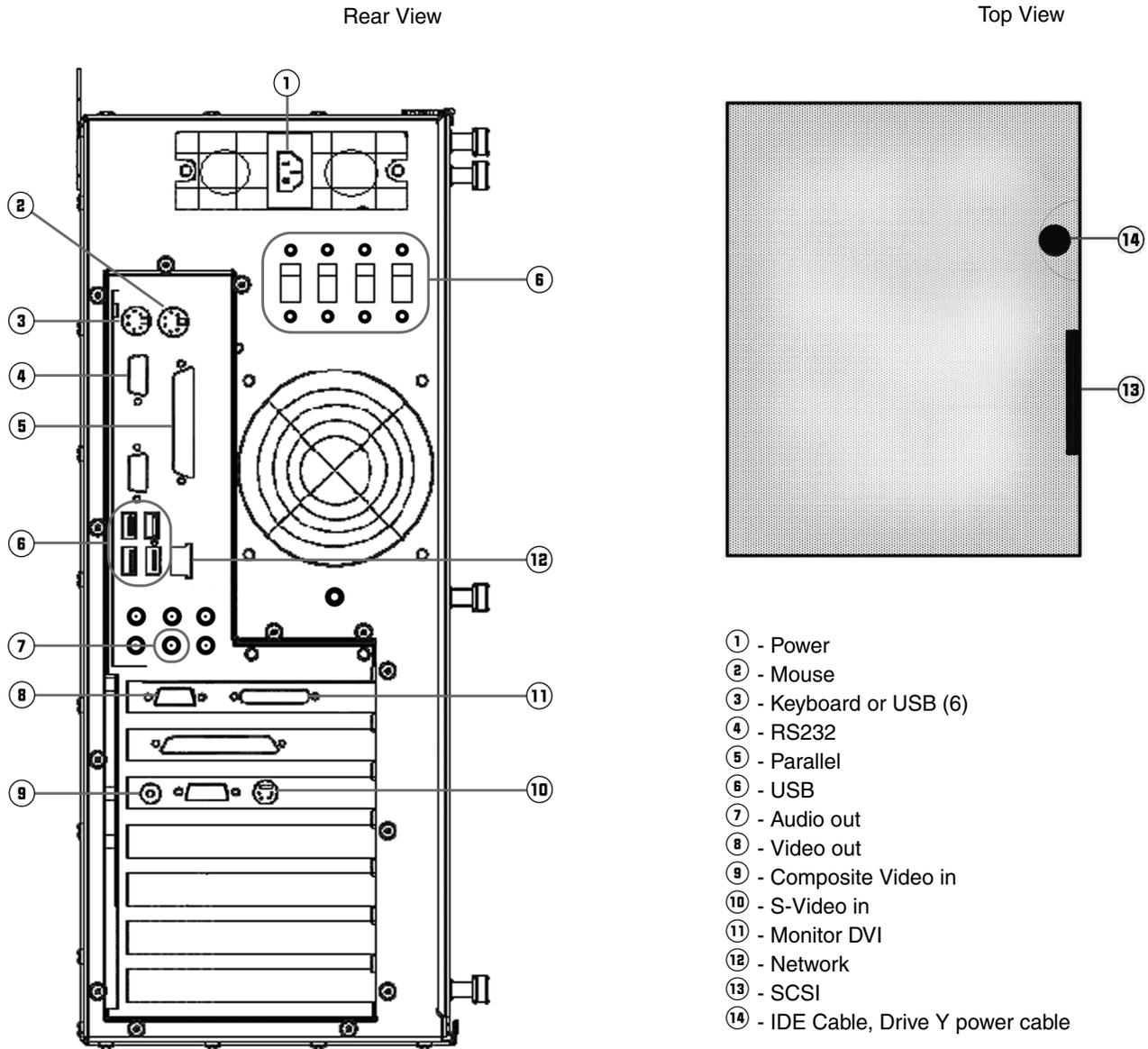
**Figure 5-4.** Ports for computer B
