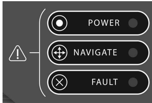
**Figure 5-7.** AXIEM™ system LED label
