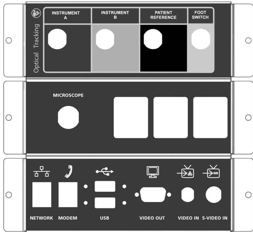
**Figure 3-1.** System I/O panels
